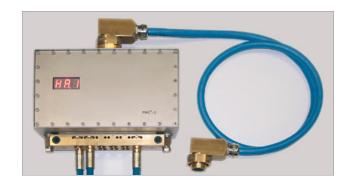
The intrinsically safe HBT PMC-D control is used on shearer or plow faces to provide high level AFC (armed face conveyor) and plow automation. Each Drive unit needs to be equipped with one PMC-D control unit and equivalent I/O to operate the CST drives or UEL gearbox functions.
