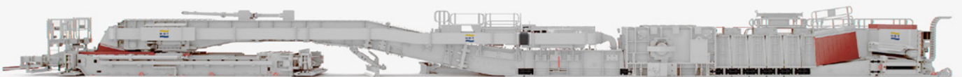
Complete HBT entry conveyor or beam stageloaader (BSL) including crusher and belt tail piece
