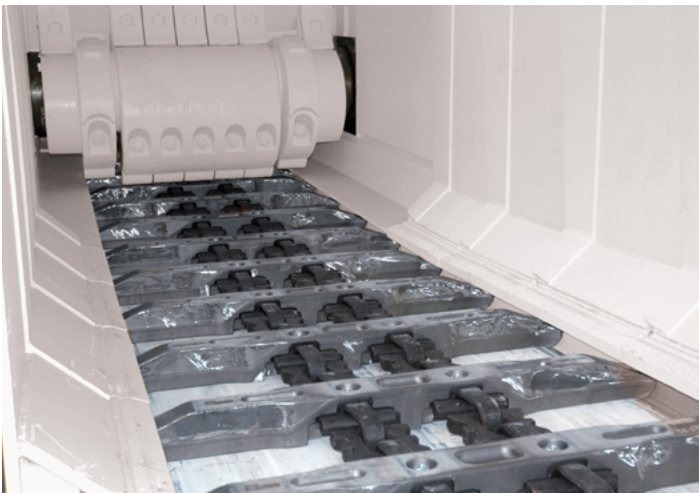
PowerChain inside a HBT BSL in the crusher area
