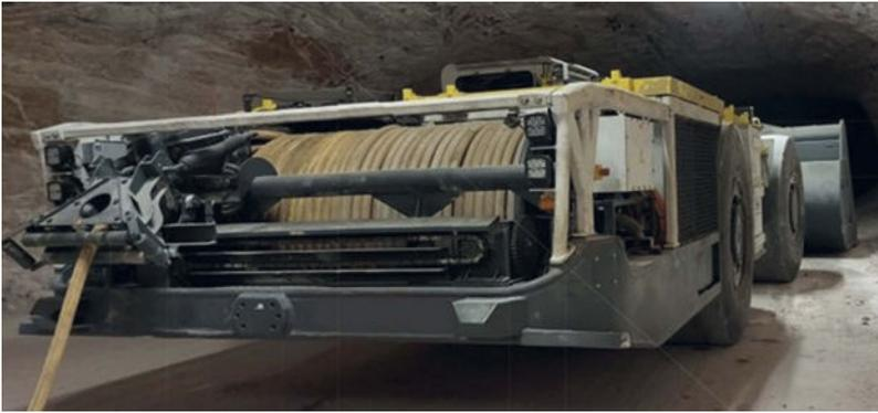
**Fig. 3:** GHH LF 19EB LHD loader with cable drum
