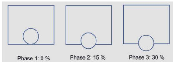
**Fig. 12:** Different entrenchment depths used in the underground test site
