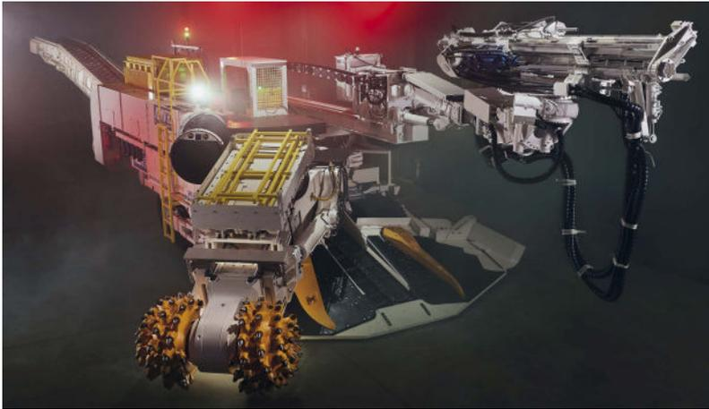
**Fig. 2:** The TDR 100 has a cutting performance of 300 kW (option to upgrade to 400 kW). The cutting arm feed is 600 mm. Various attachments can be fitted, such as the roofbolt drilling and setting device shown here.
