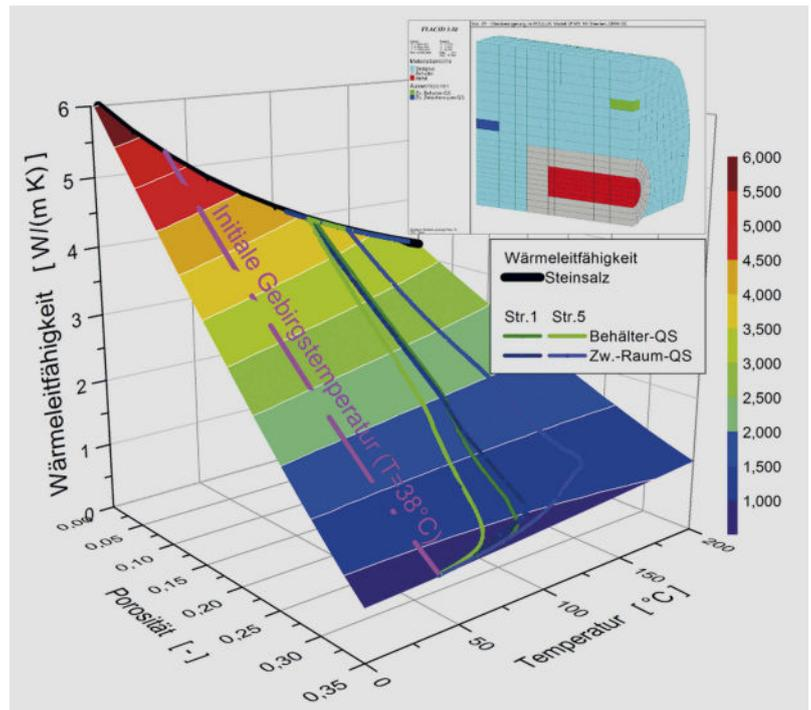
**Fig. 1:** The relation between thermal conductivity depending on the porosity and the temperature [1]
