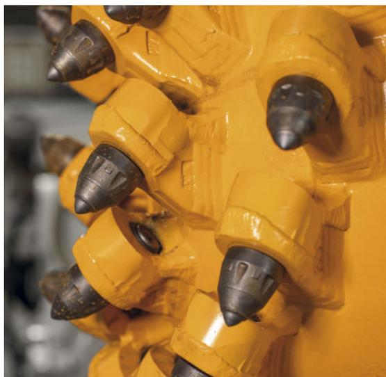
**Fig. 3:** Every TDR machine – from the smallest to the largest – has been developed from the ground up to cope with the highest stresses that arise in the harsh underground environment. Here a close-up of the cutting head.
