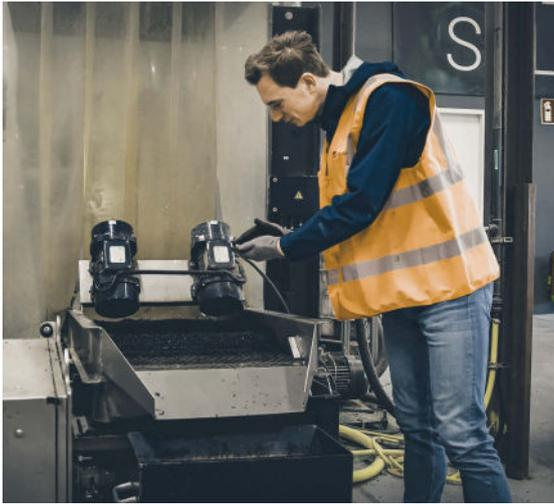
**Fig. 3:** Transformation of recycled geotextile into pellets for reuse
