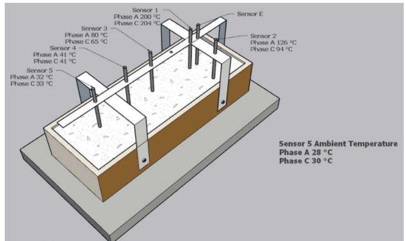
Fig. 16: Laboratory experiment sensors' readings comparison between Phases A and C after three hours of operating
