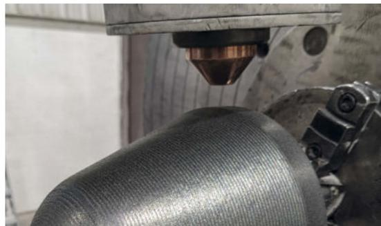
**Fig. 2:** Wear parts like this stone crusher tooth with an outer diameter of about 140 mm are re-stored with the LMD process. Thanks to AI, the processes for repairing irregular surfaces shall be optimized.
