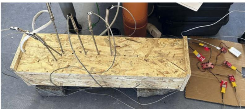
**Fig. 6:** Beta model setup showing the heating setup and the logging system connected while performing the test
