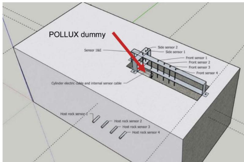
**Fig. 18:** 3D-visualization of recommended model for future research
