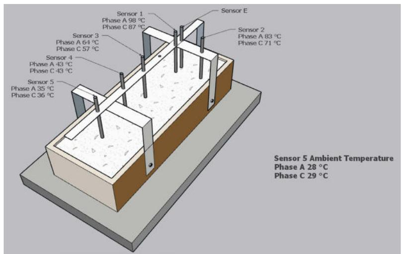
Fig. 17: Laboratory experiment sensors' readings comparison between Phases A and C after one hour of cooling down
