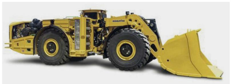
**Fig. 7:** Komatsu WX 22H LHD loader with hybrid drive
