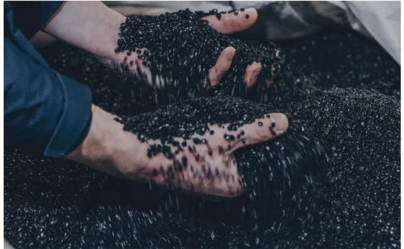
**Fig. 4:** Pellets prepared from recycled geotextile, ready for integration into new geosynthetic products
