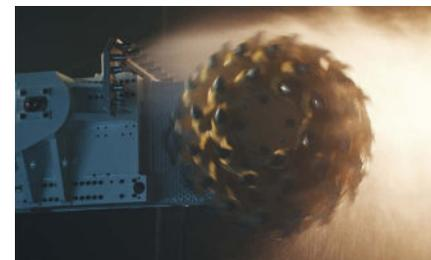
**Fig. 5:** The highly effective water spray system (water curtain sprays) shown in action at the cutting head. This has been designed to reduce water consumption and efficiently suppress dust production.
