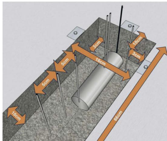
Fig. 10: In-situ experiment model showing the sensors’ placement position and model dimensions
