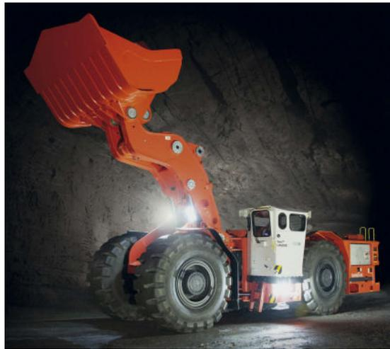
Fig. 12: Toro LH 625 IE LHD loader with supply cable
