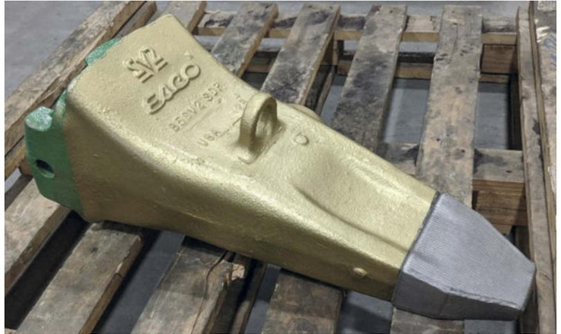
**Fig. 1:** The AI tool developed as part of the AI-SLAM project speeds up the laser coating and repair of components with complex geometries (pictured: a blade tooth)
