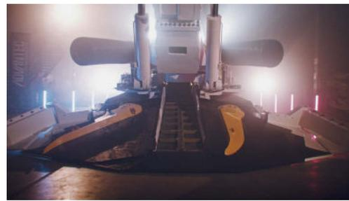
**Fig. 1:** Structural symmetry keeps vibration levels down when the machine is cutting and loading.
