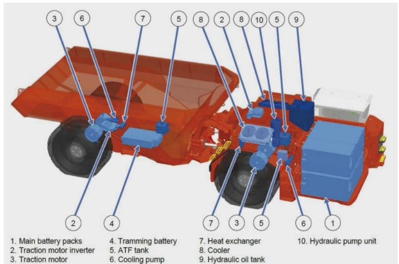
**Fig. 6:** Sandvik TH665 B dump truck with four wheel traction motors
