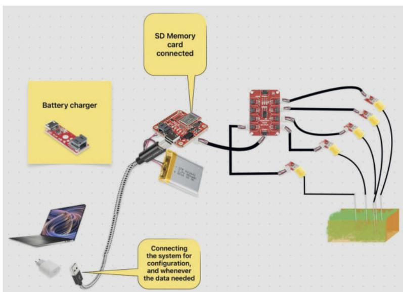
**Fig. 3:** Logging system setup
