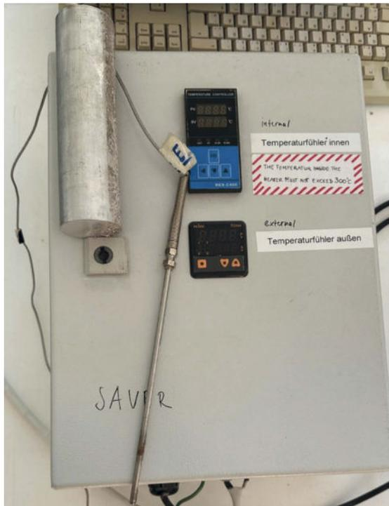
**Fig. 2:** Heating setup showing the miniature POLLUX (left) and heating controller
