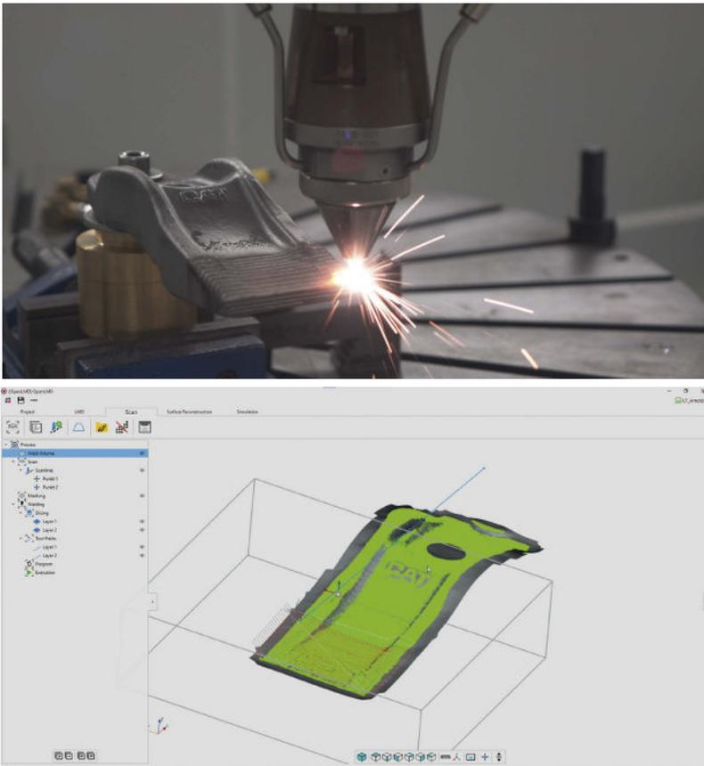
**Fig. 3:** The AI-driven LMD process simplifies the operator's role in coating excavator teeth.
