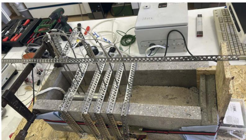
**Fig. 14:** Laboratory experiment model showing the sensor placement position and model dimensions (before backfill was filled)
