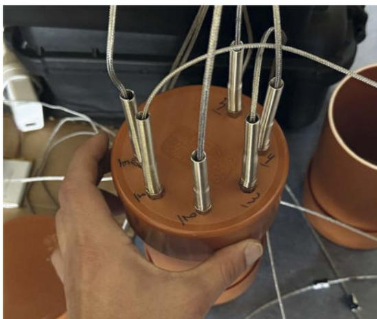
**Fig. 4:** Logging system water pre-test. The tube contains the hot water and the cover holds the sensors while logging the readings.
