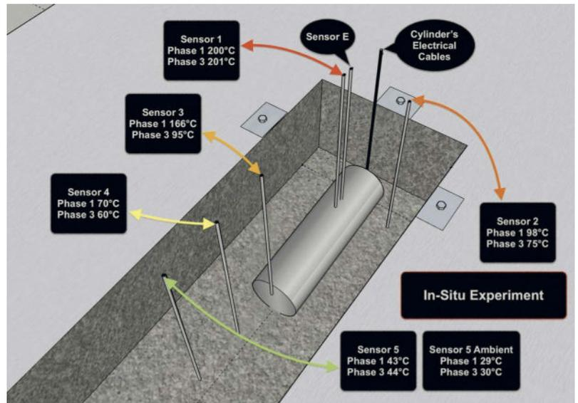
Fig. 15: In-situ experiment sensors' readings comparison between Phases 1 and 3 after eight days of operating
