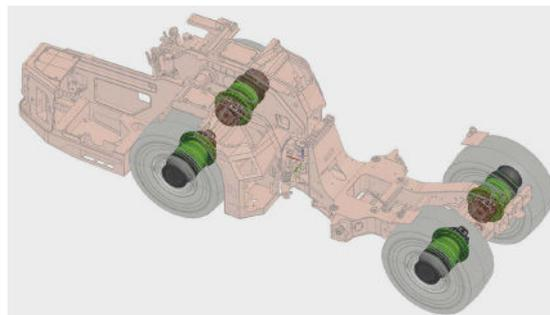
**Fig. 9:** Sandvik battery powered dump truck with traction motors
