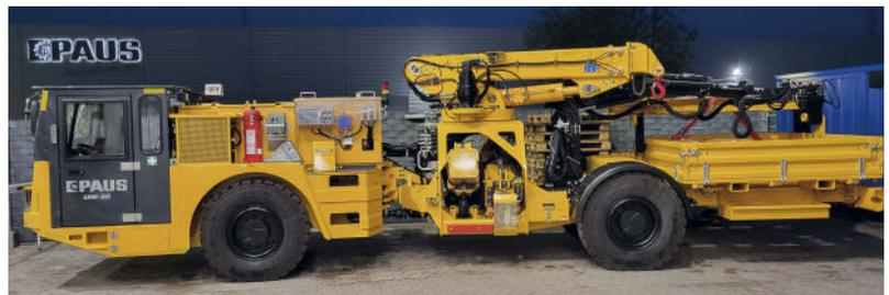
**Fig. 8:** Service truck with the latest diesel technology – Paus Uni 50 LP-IH (Idler Handler)
