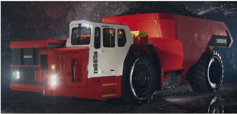
**Fig. 10:** Sandvik TH665 B dump truck with battery changeover system
