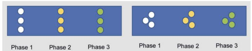
Fig. 8: Pre-testing with linear (left) and triangle (right) positioning of the sensors
