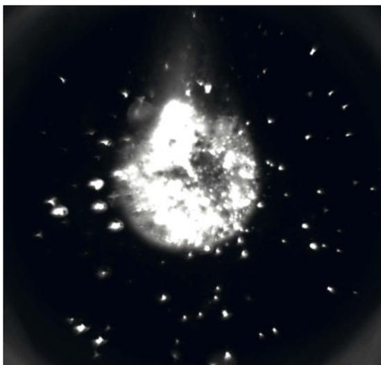
**Fig. 5:** Coaxial weld pool image from laser metal deposition in the AI-SLAM project
