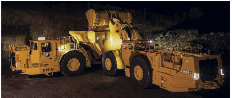
Fig. 13: Caterpillar R 2900 XE LHD loader with battery unit
