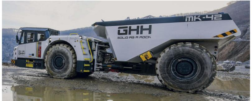
**Fig. 1:** GHH MK-42 dump truck fitted with the latest diesel technology in Tier 3 and Tier 4 final version with Stage V upgrades
